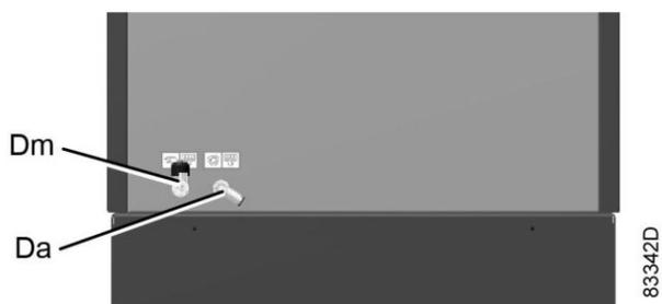
Condensate drain connections, typical example
