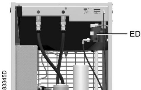
Location of electronic water drain (Workplace)
