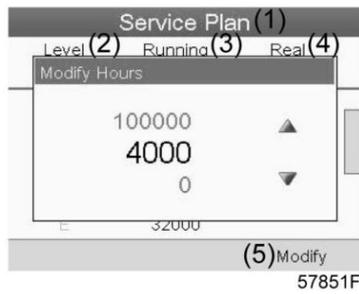
Modify the value as required using the ↑ or ↓ scroll key and press the Enter key to confirm.
