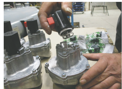
Remove the twist-on coil from the solenoid.
