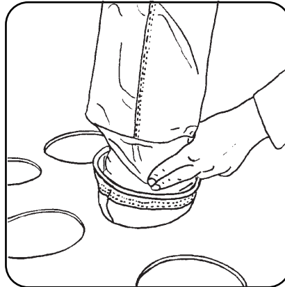
Fig. 1. Fit the collar into the hole and then push the bag through the collar. Do not remove the collar until the bag is all the way through.
