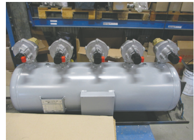
Fit the twist-on coil on the solenoid. It should face right when looking at the air receiver from the fitting plate side..
