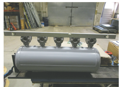
Check that all solenoid valves are level using a spirit gauge.
