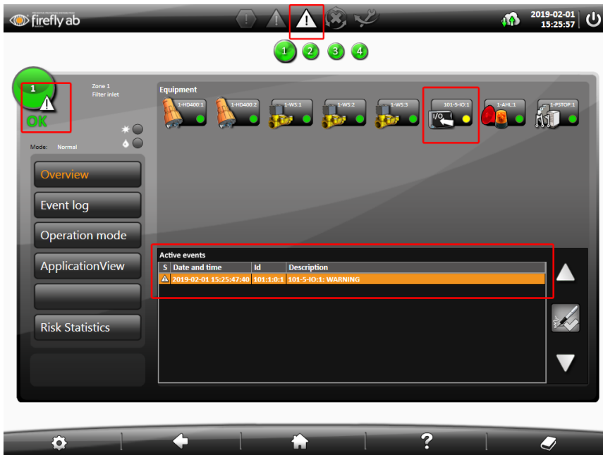
Figure 8 Event for warning on digital input
