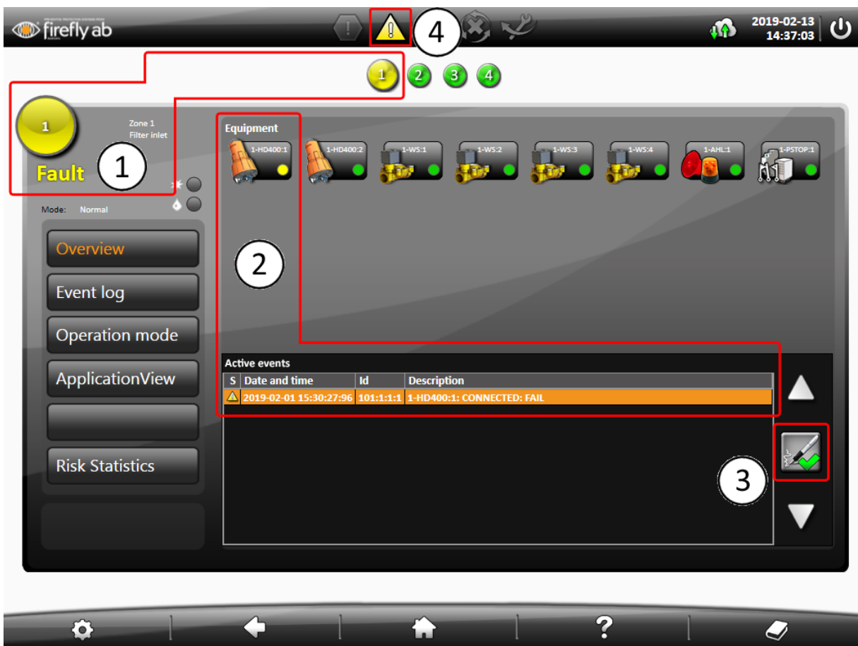
Figure 9 Event for detector fault
